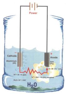
As Tap water contains a certain amount of dissolved salts it is able to conduct current when the power is turned on. This causes one of the two electrodes to dissolve in the water resulting in a colour change in the water and the formation of visible particles.
